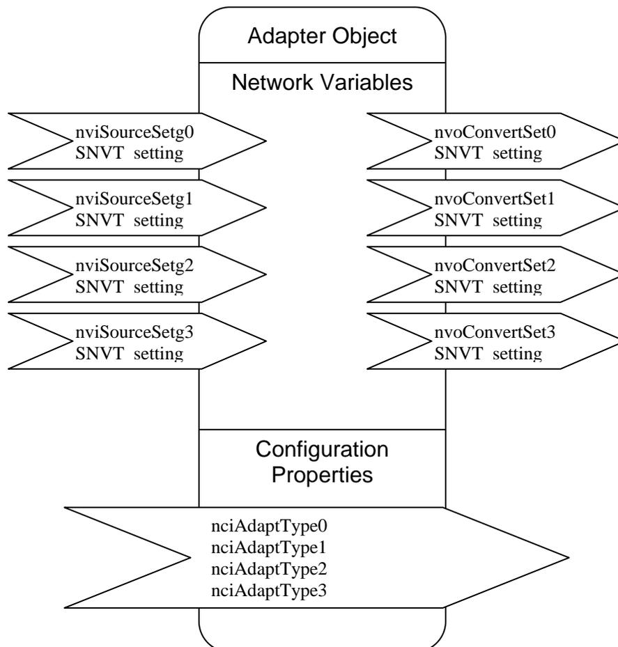
Figure 2 Functional-Block Details
