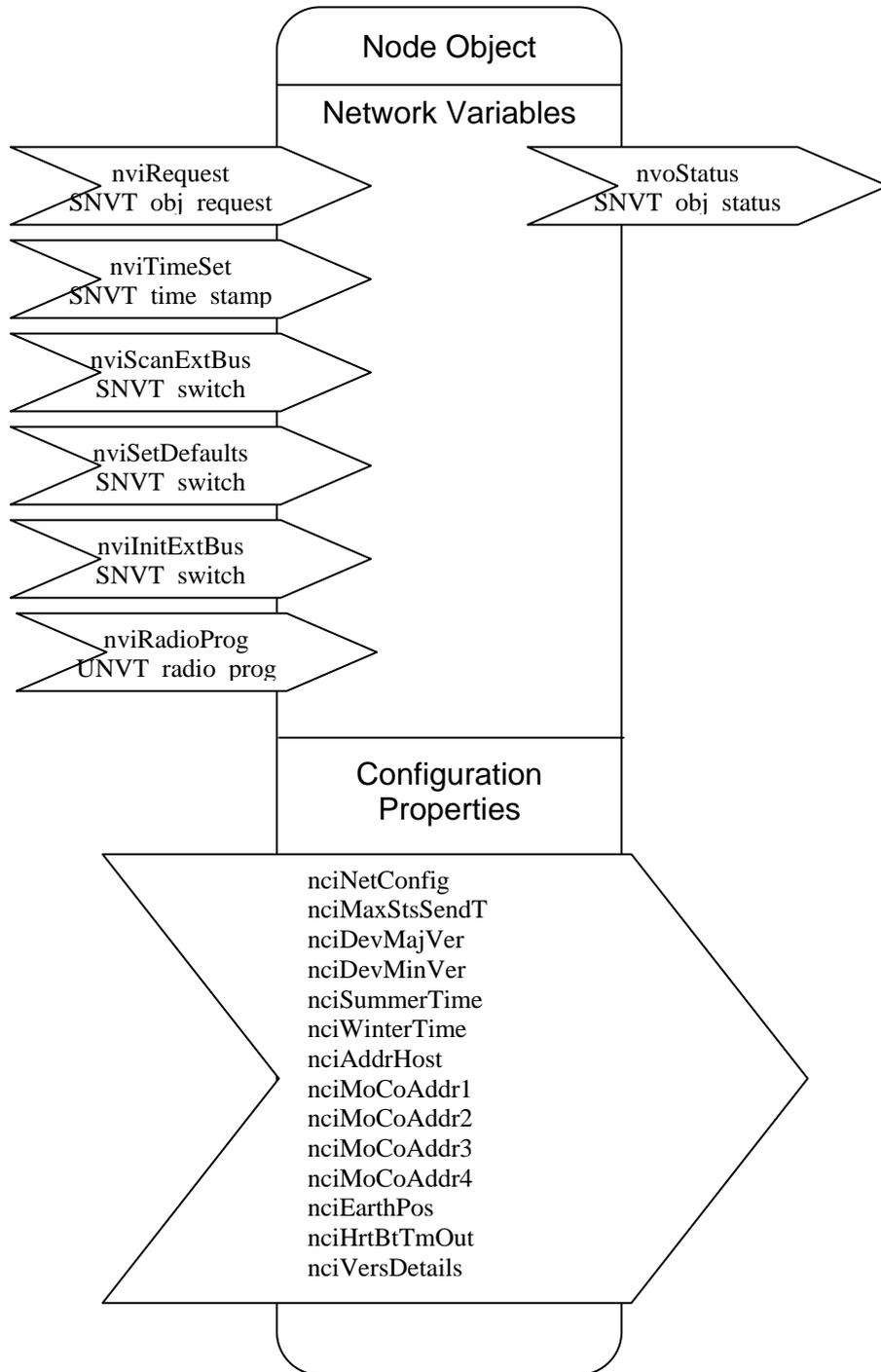
**Figure 2** Functional-Block Details
