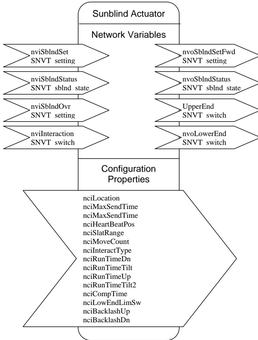
**Figure 2** Functional-Block Details
